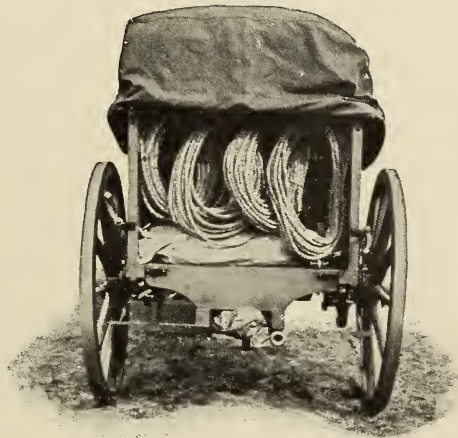
FIG. 97.—Wagon carrying tools and appliances, the balloon being packed on the top.
