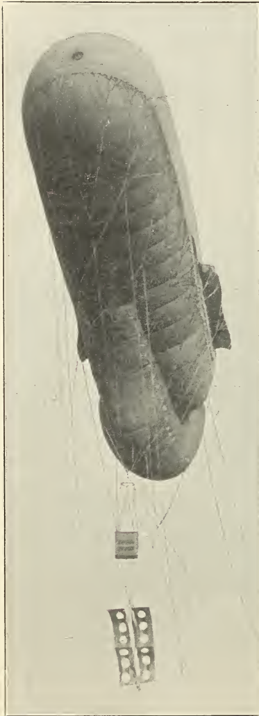
FIG. 115A.—The kite-balloon designed by Major von Parseval and Major von Sigsfeld.
