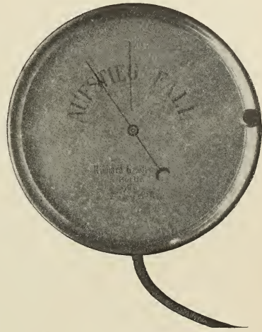
FIG. 17.—The statoscope, by Gradenwitz.
