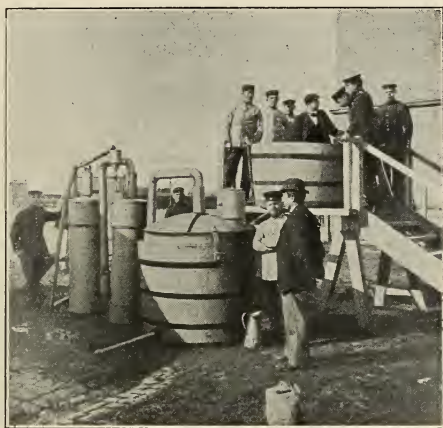
FIG. 147.—Apparatus for generating hydrogen.
