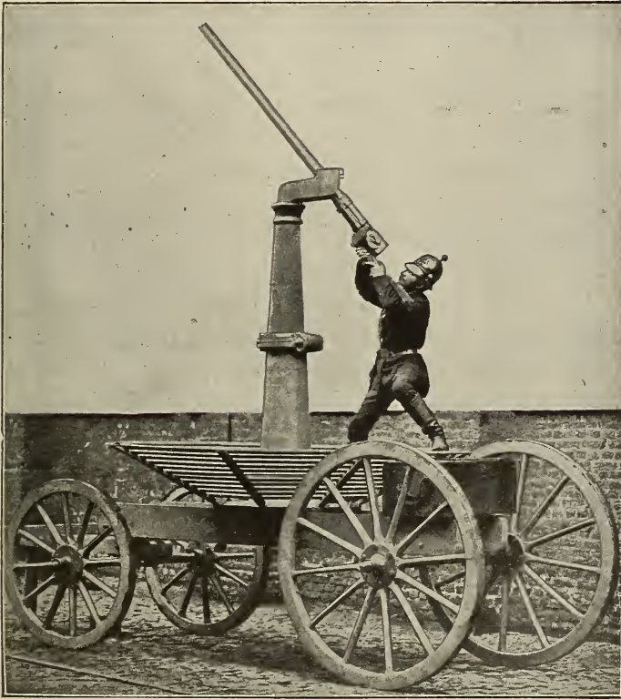
FIG. 89.—Gun constructed by Krupp for firing at balloons.
