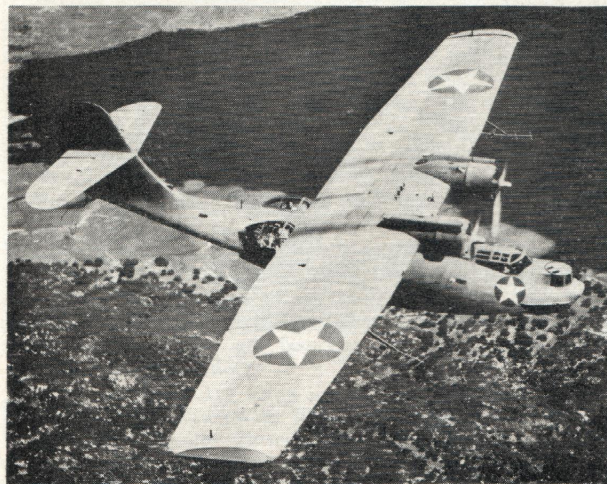
Top: A PBY-5A with red rudder striping and early US Navy wartime camouflage. She retains the red centre to the stars. Above: A standard PBY-5 of the US Navy, complete with ASV aerials on its wing leading edges, and grey/blue paintwork.
